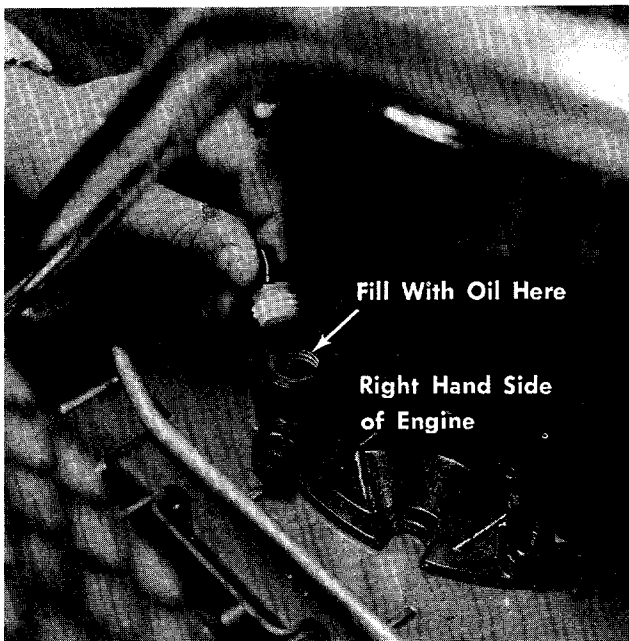
FIGURE 27. OIL FILL LOCATION
